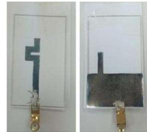
Fig. 2: The proposed antenna design printed on glossy paper
